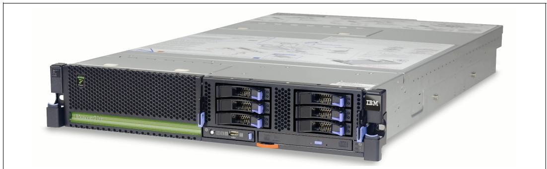
Figure 1-1 IBM Power 710 server
